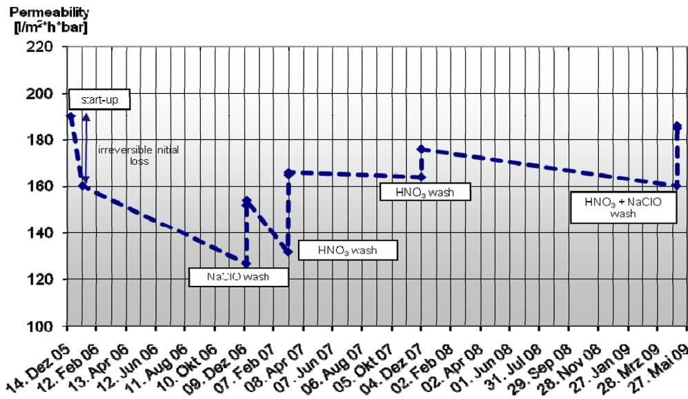
Figure 6: Stable conditions using acid recovery wash
