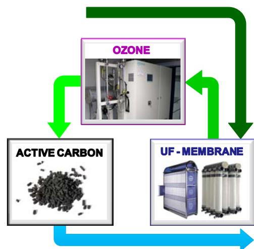
Picture 3b: 3-stage MBS for higher loaded surface water
