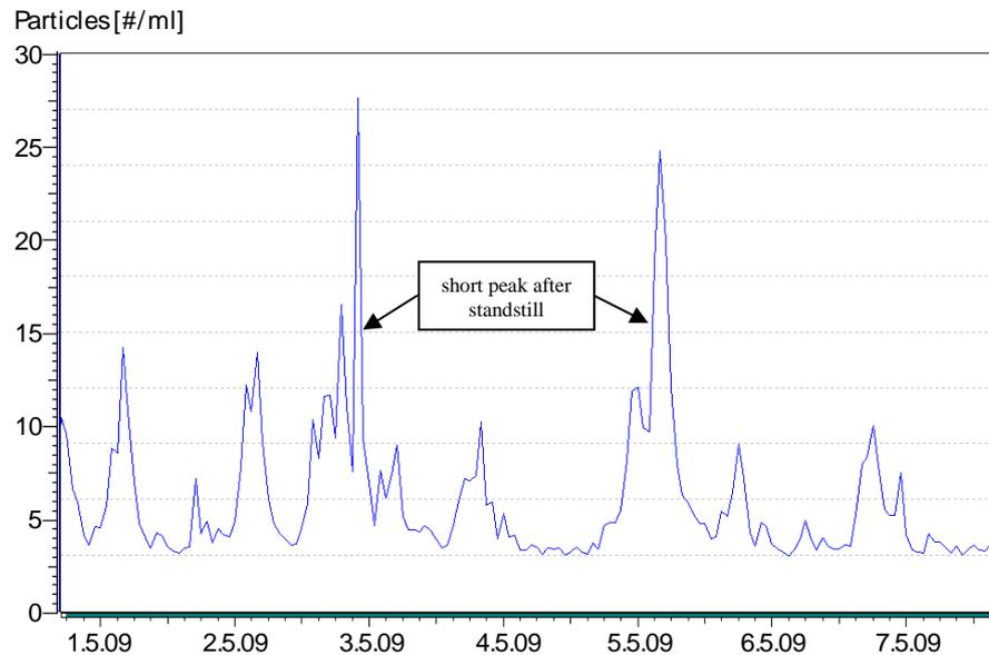
Figure 4: Typical total particle count in permeate
