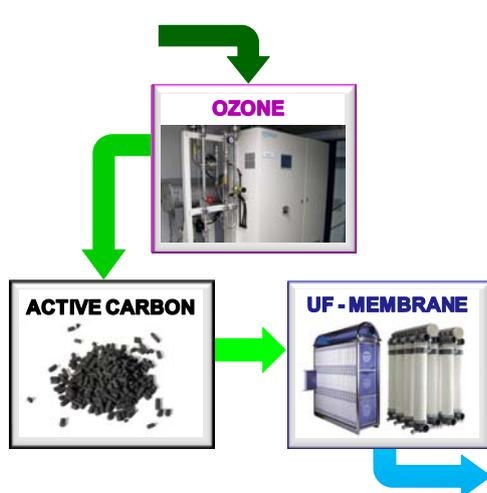
Picture 3a: 3-stage MBS for lower loaded surface water
