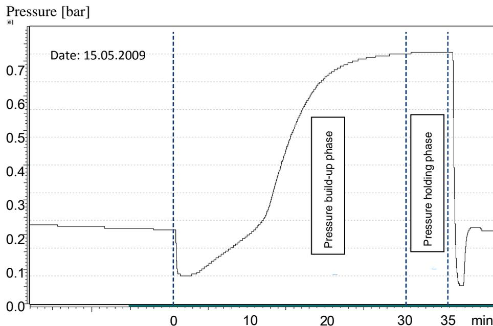
Figure 5: Integrity test on rack with 41 modules – 2000 m<sup>2</sup> filtration surface
