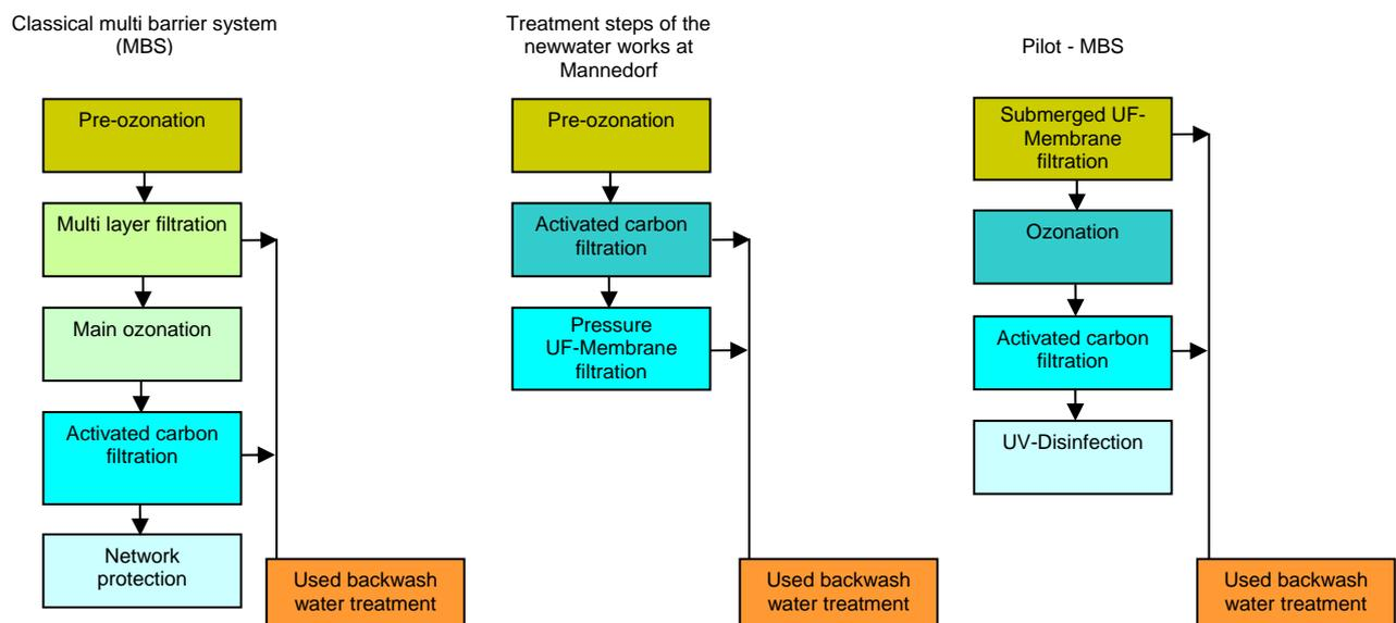
Figure 1: Process development for the treatment of surface water
