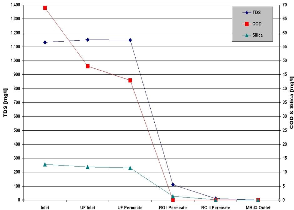
Figure 3. Removal of TDS, COD and silica – Panipat reclamation plant
