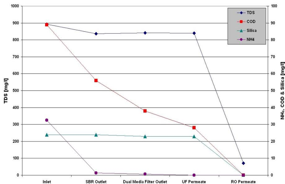
Figure 5. Removal of TDS, COD,  $\text{NH}_4$  and silica – Chennai reclamation plant
