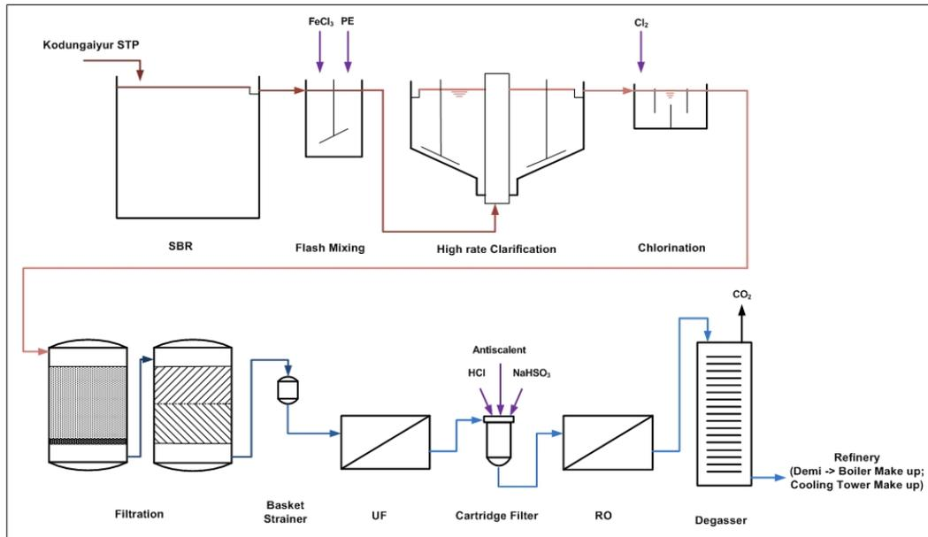
Figure 2. Chennai water reclamation and reuse process diagram
